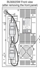
Cooling Fan Model: BUF3002S \* Different model from the rear cooling fan
